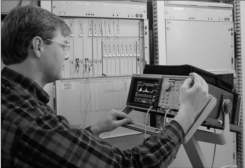
The CTS 710 SONET Test Set is the ideal tool for installing, commissioning, and provisioning SONET rings.
